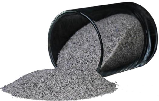
Monocrystalline Alumina is manufactured in an electric arc furnace using a selective grade of alumina with special additives. The unique processing method makes these self-sharpening grains with superior cool cutting and grinding required for abrasive applications.
