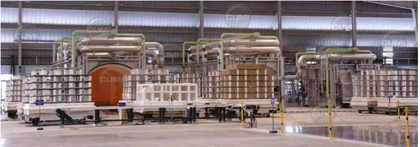
Batch Kilns with operating Temp. upto 1750°C
