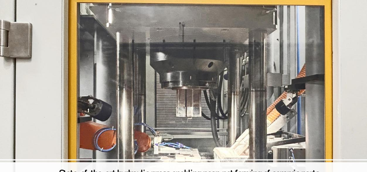
State-of-the-art hydraulic press enabling near-net forming of ceramic parts
