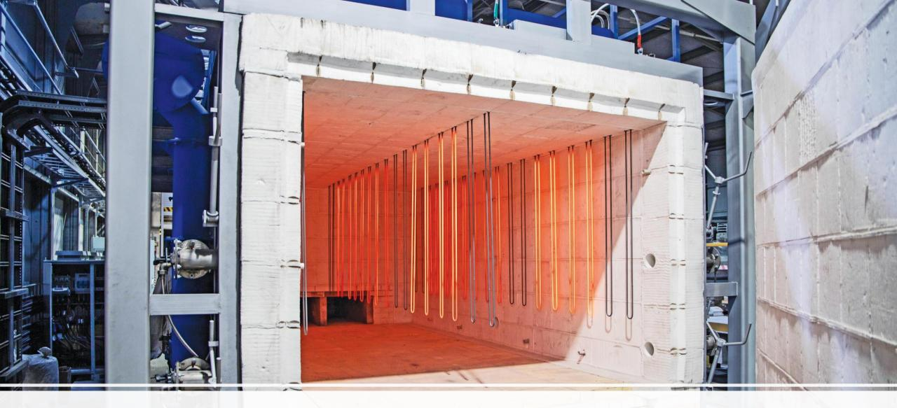
Kiln commisioned at VAWRussia to increase the Ntride Bonded Silicon Carbide capacities
